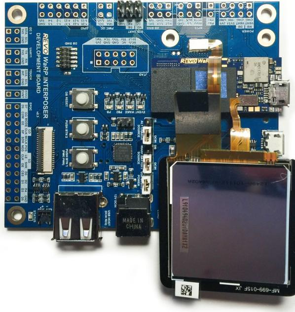
If the touch controller is not encapsulated, cover exposed contacts with electrical tape to avoid shorting to WaRP.
